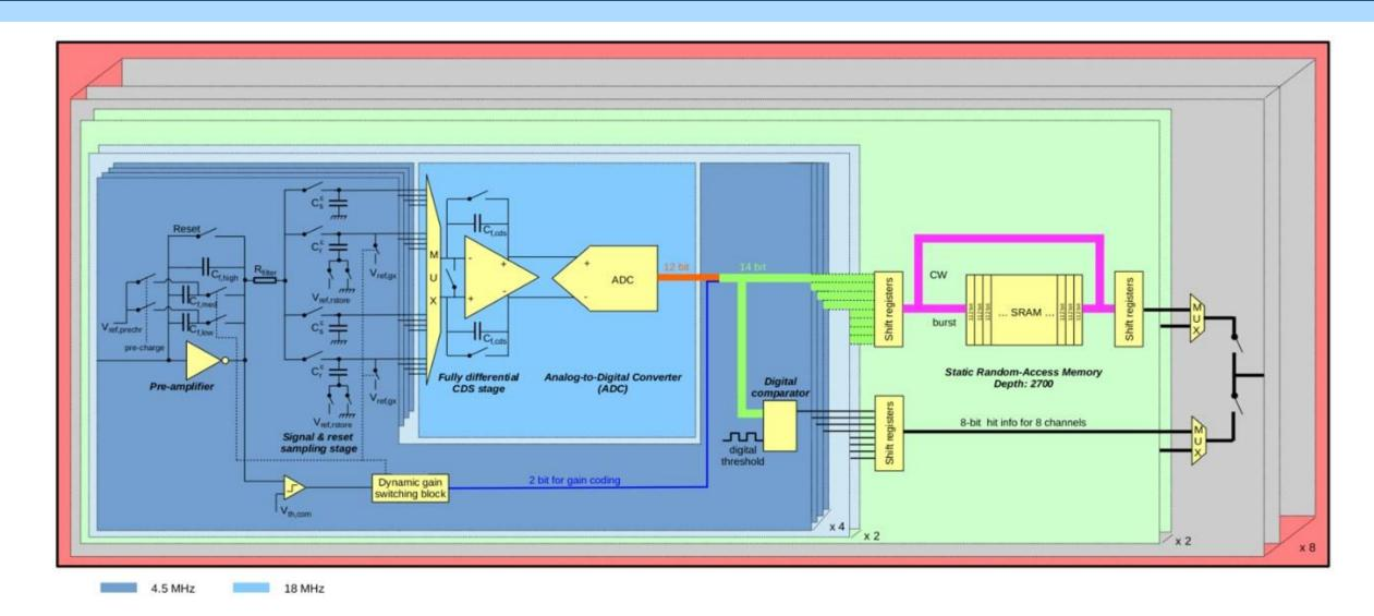
Simplified block diagram of the GOTTHARD-II chip [1]. Thanks to its on-chip ADCs (Analogue-to-Digital Converter), it provides 4.5 MHz frame rate allowing for real time analysis of the X-ray beam profile
