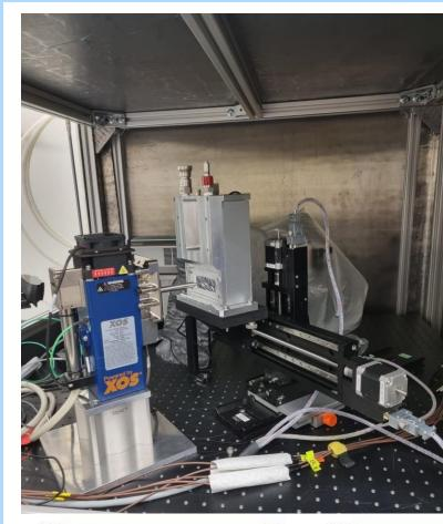
First tests on 20um detectors were carried out on a compact X-ray generator (@ SuperXAS) with a Mo anode where the beam is focused with polycapillary optics to a 50 µm at 20 mm from the optics. A 2D scan with a 150 μm step size on the X axis and 40 μm on the Y axis was performed, acquiring 1000 frames (frame rate 2.5 MHz, exp. time 100 ns) of the 256 pixels at each position of the scan in dark and under illumination conditions in order to subtracts the pedestal level from the data.
